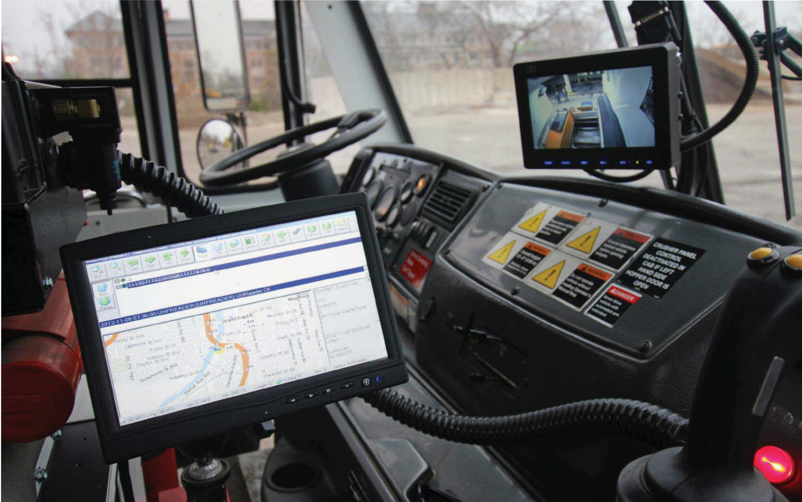
The RFID-enabled trash-collection system monitors which residents have paid for service.
